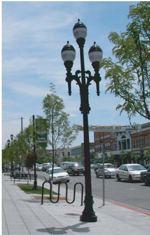
DECORATIVE LIGHT POLE MODEL: Mountain States Lighting #16TFS-7-5/16S-20" LIGHT FIXTURE MODEL: Hadco part #S8494Y-165 Induction w/ photocell receptacle BANNER POLE MODEL: Mountain States Lighting #15SRS-4.0
