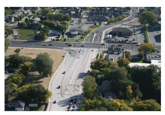
Figure 2-18 Continuous Flow Intersection
