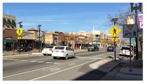
Figure 4.13 Rapid Rectangular Flashing Beacons in Ogden, UT
