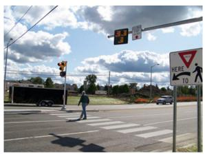
Figure 4.14 Typical Hybrid Pedestrian Crossing
