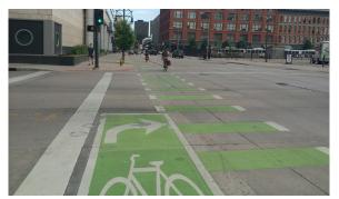
Figure 4.17 Typical two-stage turn queue box
