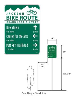
Figure 4.20 Typical Bikeway Wayfinding Signage
