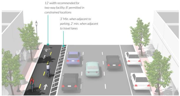
Figure 4.8 Typical Two-way Protected Bike Lane
