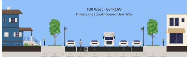
Figure 4.25 Possible 100 West Couplet-scenario cross-section
